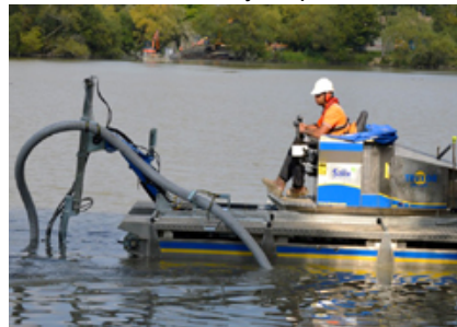
The versatile and manoeuvrable Truxor performs a wide range of river maintenance tasks including pump desilting
